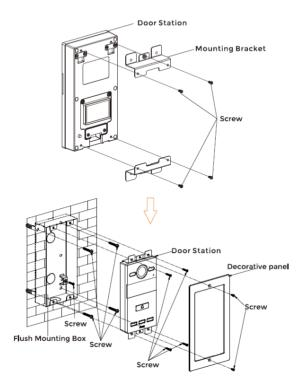
Product size:  $88 \times 168 \times 32.5 \text{ mm}$ Flush Mounting size:  $120 \times 210 \times 48 \text{ mm}$ Hole-cutting size:  $98 \times 199 \times 42 \text{ mm}$
