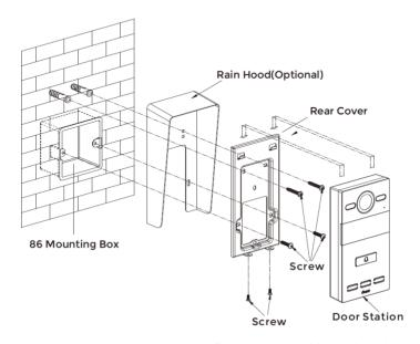
Product size:  $88 \times 168 \times 32.5 \text{ mm}$ Surface Mounting size:  $88 \times 168 \times 34 \text{ mm}$
