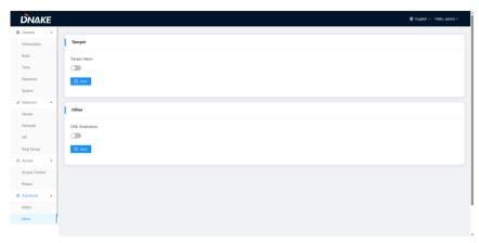
Tamper Alarm: Enable to use Tamper alarm on the back of the device;
