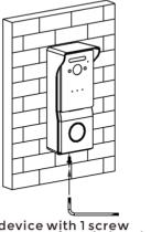
Lock the device with 1 screw (different screws for rain hood and bracket).
