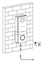
12. Use wrench to lock the bottom of the device with 1 screw (different screws for rain hood and rear cover).
