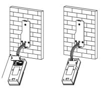
10. Fix interface clamp to the device with 2 screws.
