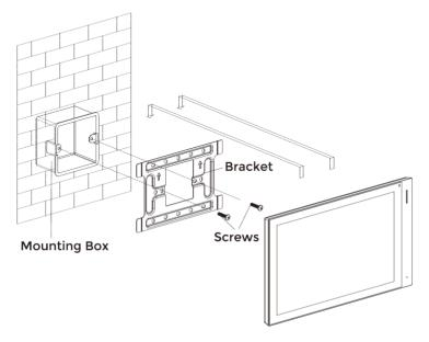
Product size:  $264.3 \times 160 \times 11.8 \text{ mm}$ Surface Mounting size:  $264.3 \times 160 \times 21.6 \text{ mm}$
