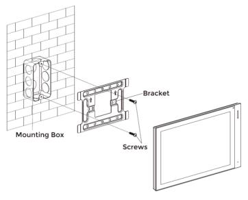
Product size:  $264.3 \times 160 \times 11.8 \text{ mm}$ Surface Mounting size:  $264.3 \times 160 \times 21.6 \text{ mm}$
