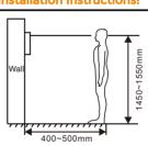
[Suggestion]: The camera should be 1450~1550mm above the ground. The camera at this height can capture human face perfectly.
