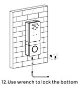
of the device with 1 screw (different screws for rain hood and bracket).
