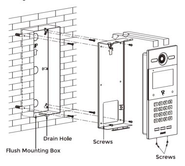
Product size:  $133 \times 295 \times 41$  mm Flush Mounting size:  $133 \times 295 \times 63.5$  mm Mounting hole size:  $124 \times 289 \times 56$  mm
