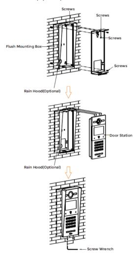
Product size:  $133 \times 295 \times 41$  mm Flush Mounting size:  $133 \times 295 \times 63.5$  mm Mounting hole size:  $124 \times 289 \times 56$  mm
