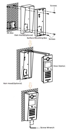
Product size:  $133 \times 295 \times 41 \text{ mm}$ Surface Mounting size:  $133 \times 295 \times 43 \text{ mm}$
