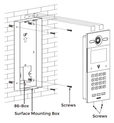
Product size:  $133 \times 295 \times 41$  mm Surface Mounting size:  $133 \times 295 \times 43$  mm
