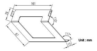
Assemble the hooks on two sides of the bracket into the groove on the rear cover of the monitor.
