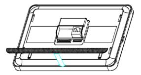
Align the edge of the silicone non-slip mat to the back of Indoor Monitor.
