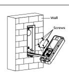
8. Fix interface clamp to the device with 4 screws
