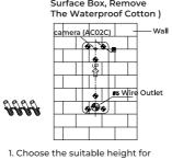
AC01/AC02. For AC02C, select the appropriate camera height. Then put the label sticker on the wall. 2. According to the sticker, drill three 8 x 45mm for screws and one 5mm for wire outlet. 3. Insert 4 screw fixing seats into the screw holes
