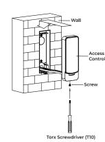
9. Use screwdriver to lock the bottom of the device with 1 screw.
