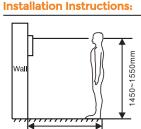
[Suggestion]: For AC02C, the camera should be 1450~1550mm above the ground.
