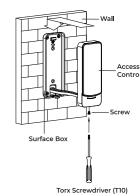
10. Hang up device with surface box. 11. Use screwdriver to lock the bottom of the device with 1 screw
