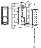
9. Neatly coil and tuck the excess wiring into the surface box. 10. Align the square slot at the top of the back cover with the clip on the box, then slide it downward until it clicks into place. 11. Secure the access control unit to the surface box by fastening the screws at its bottom
