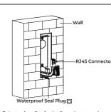
5. Let wires(included) and network cable without RJ-45 plug go through rain hood and waterproof seal plug. 6. Connect RJ-45 Plug.
