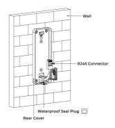
6. Let wires(included) and network cable without RJ-45 plug go through rear cover and waterproof seal plug.
