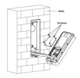
8. Fix interface clamp to the device with 4 screws.
