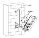
8. Fix interface clamp to the device with 4 screws.
