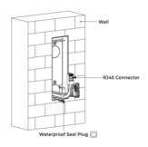
5. Let wires(included) and network cable without RJ-45 plug go through rain hood and waterproof seal plug.
