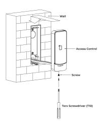
9. Use screwdriver to lock the bottom of the device with 1 screw
