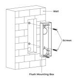
4. Lock the Flush Mounting Box with 2 screws.
